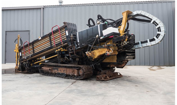
Photograph of a typical drilling rig used to install horizontal wells. This drill rig is capable of installing horizontal wells extending as much as 1,000 feet from the surface location and thus eliminates the need to disturb surface activities.
